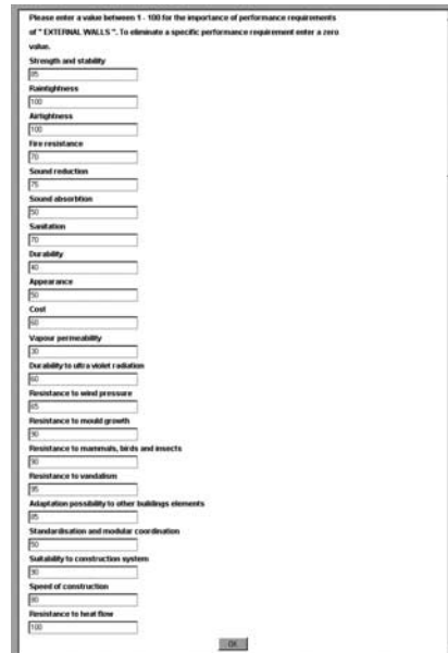
Figure 2D. User dialog boxes in BES. (The list for the performance requirements of external walls with editable default values.)
